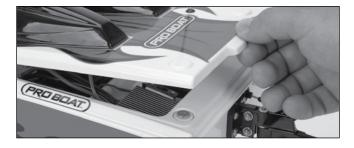
Make sure the receiver switch is in the "OFF" position. Install a fully charged 7.2V Ni-MH battery pack into the radio box. Follow the
