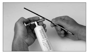
**Note:** Running the Apache 24 EP RTR in salt water could cause some parts to corrode. If you run the boat in salt water, rinse it thoroughly in fresh water after each use and lubricate the drive system.
