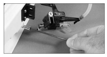
5. Lubricate the drive shaft with PRB0100 Marine Grease. Reinstall the drive shaft in reverse order. Be sure to reinstall the nylon washer between the universal and the stuffing box.
