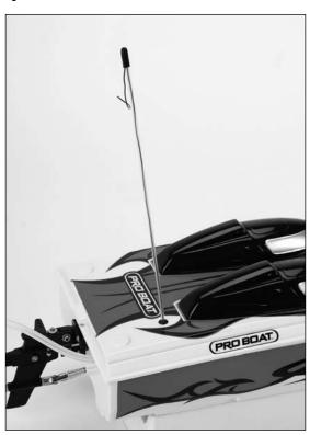
Turn the transmitter on, then the receiver. Check for correct operation. The rudder control arm should move toward the front of the boat when right input is given. Conversely, when left input is given, the control arm should move toward the back of the boat.
