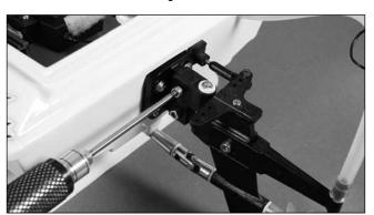
4. Move the rudder assembly and slide the drive shaft out of the stuffing box.
