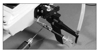
3. Remove the two 3mm screws from the outdrive to separate the rudder assembly from the mount. Make sure not to lose the 3mm nuts when removing the screws.
