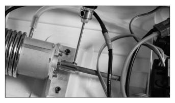
2. Loosen the 1.5mm setscrew connecting the universal joint to the drive shaft.
